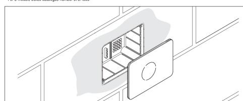
The protective cover has been designed so to protect the inside of the connector blocks during any building and painting operation.
