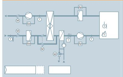
Demand-based operation of ventilation plants ensures energy-efficient ventilation. Depending on the requirements and type of plant, important plant elements that must be activated in an energy-optimized manner are outside air, exhaust air, recirculated air or bypass dampers. OpenAir damper actuators satisfy these requirements precisely and reliably.
